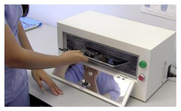
The UV Box's 55-second cycle time fits within the World Health Organization's guidelines on hand washing duration, meaning hand hygiene and device disinfection can happen simultaneously.
